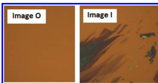
Figure 2. Microscopy images of the substrate (left panel) and FLG on substrate (right panel) obtained with 100X objective. Image O is used for the background subtraction, a required step for the large area graphene identification. Image I is used for the overall graphene layer identification experiment.
