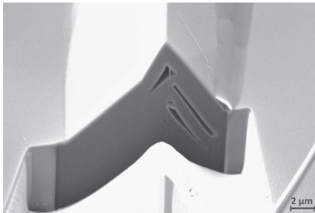
Fig. 6 Cross section of a wrinkle by Focused Ion Beam cutting
